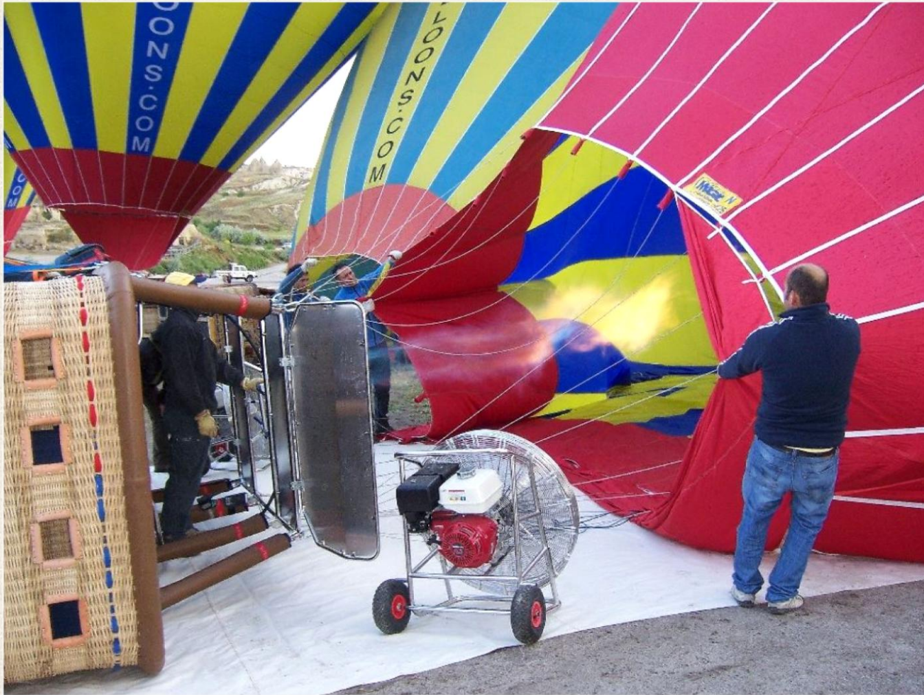
Note the fan blowing the heated air into the balloon.
