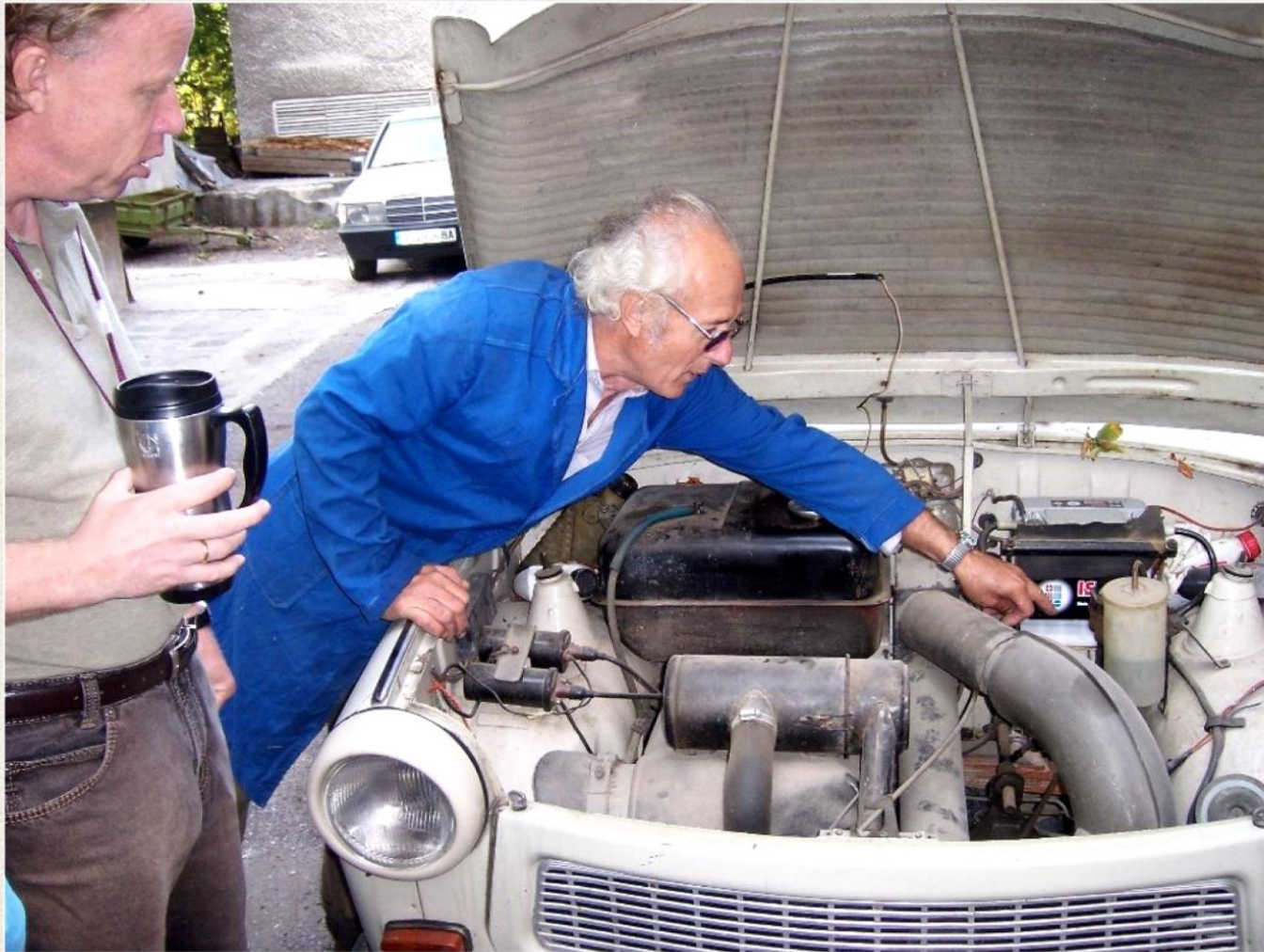
A Bulgarian man proudly showing us his car, which is a copy of an East German car. Metal was scarce in Bulgaria, so the body of the car is made of molded wood chips and glue.
